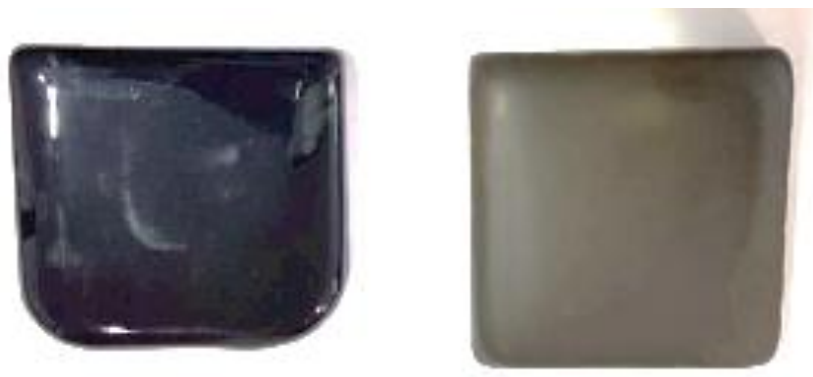
Figure 2 – Glass (left) and glass-ceramic (right) pieces obtained from the tailings.
