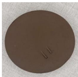
Figure 2. Sintered 50 mm-disc produced by compaction pressure of 39.2 MPa and 10% w/w starch-based ligant due to temperature change
