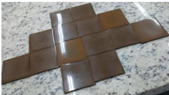
Figure 3. Sintered plates of 100 mm length x 100 mm width after polishing are displayed
