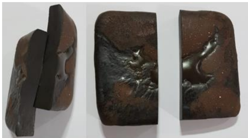
Figure 5 Crystallized glass-ceramic pieces at 850 °C obtained from melting (1400 °C) and annealing (675 °C)
